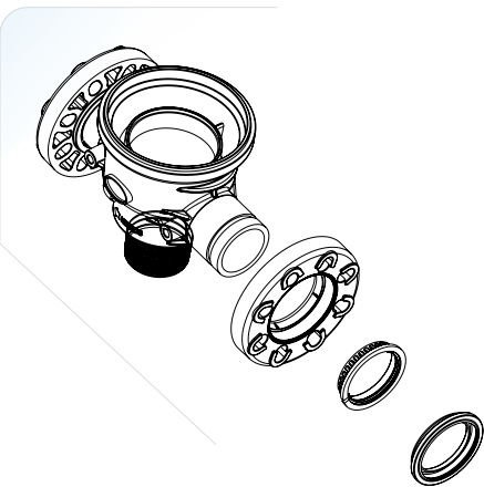
Connection Type: Victaulic/Threaded/Optionally 3" Flanged
